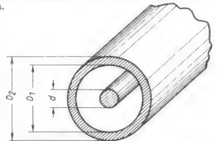
$$L = l \left( 2 \ln \frac{D_1}{d} + 2 \frac{D_2^4}{(D_2^2 - D_1^2)^2} \ln \frac{D_2}{D_1} - \frac{D_2^2}{D_2^2 - D_1^2} \right) \cdot 10^{-3} \quad \mu\text{H} \quad (6,1)$$
